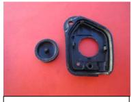
Remove old plastic button ending up with hard plastic shell ready for inserting new silicone button in.
