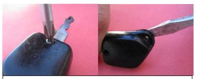
Use phillips screwdriver to unscrew remote and than prise it open with flat screwdriver on the split line.
